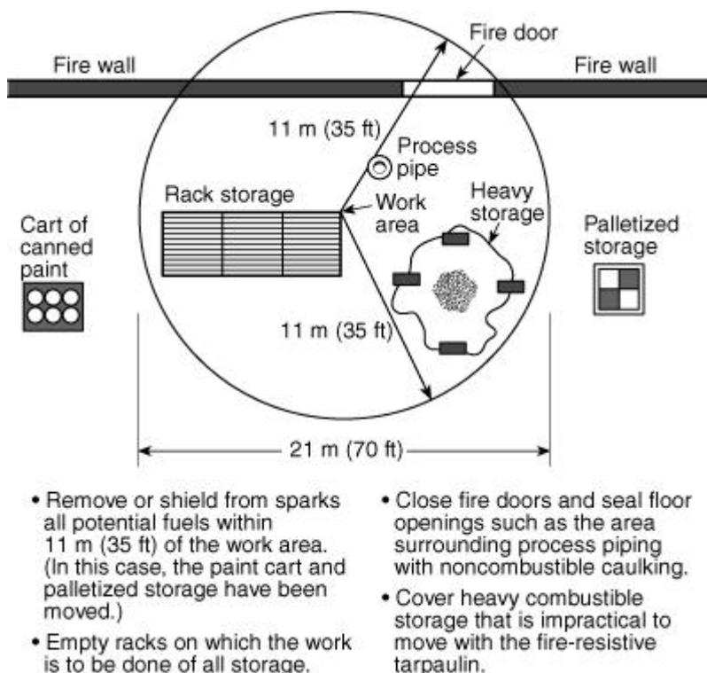
**FIGURE A.5.4.1(1) The Hot Work 11-m (35-ft) Rule. (Courtesy of Factory Mutual Engineering Corporation.)**
