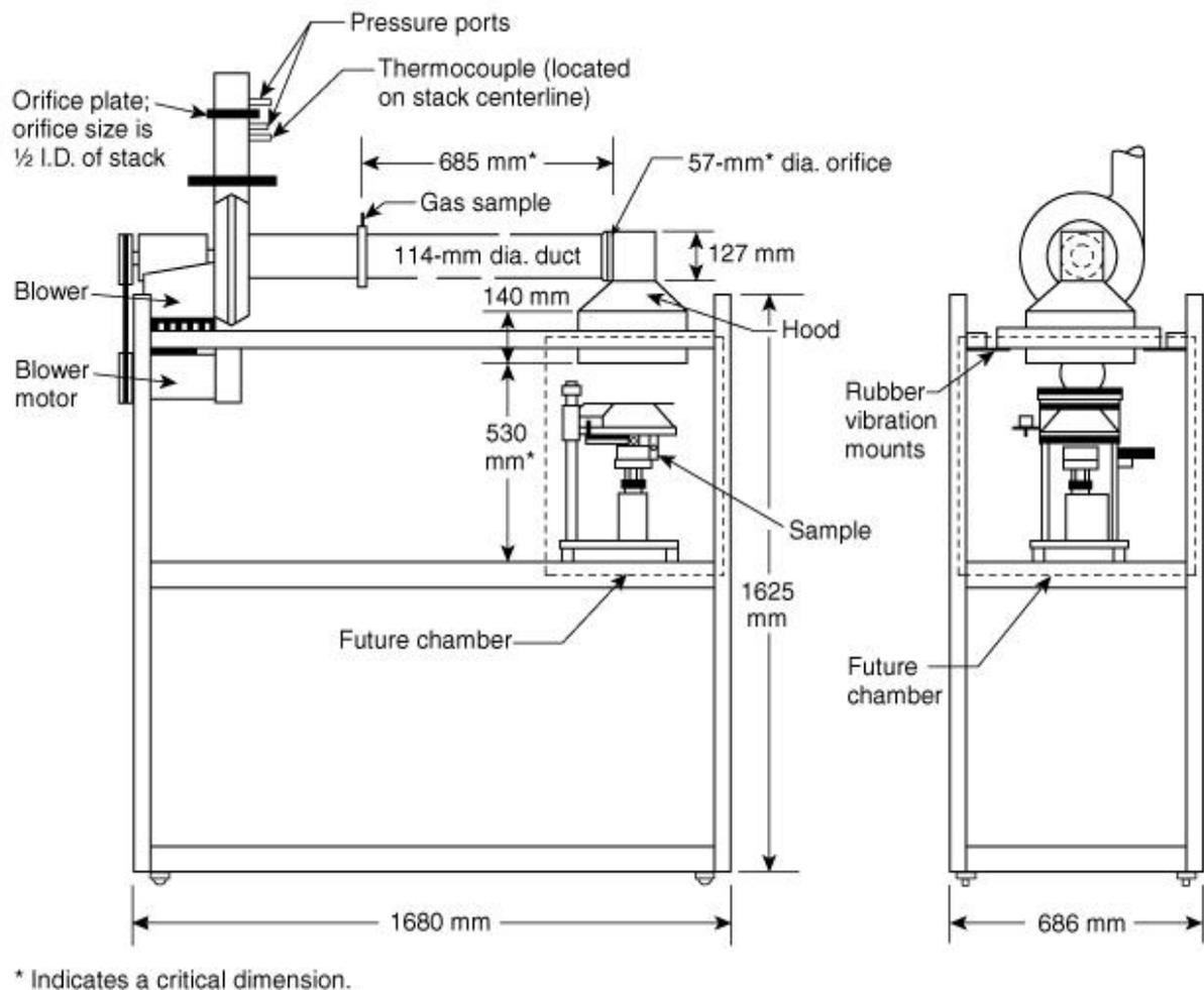
FIGURE 4.1.2 Overall View of Test Apparatus.
