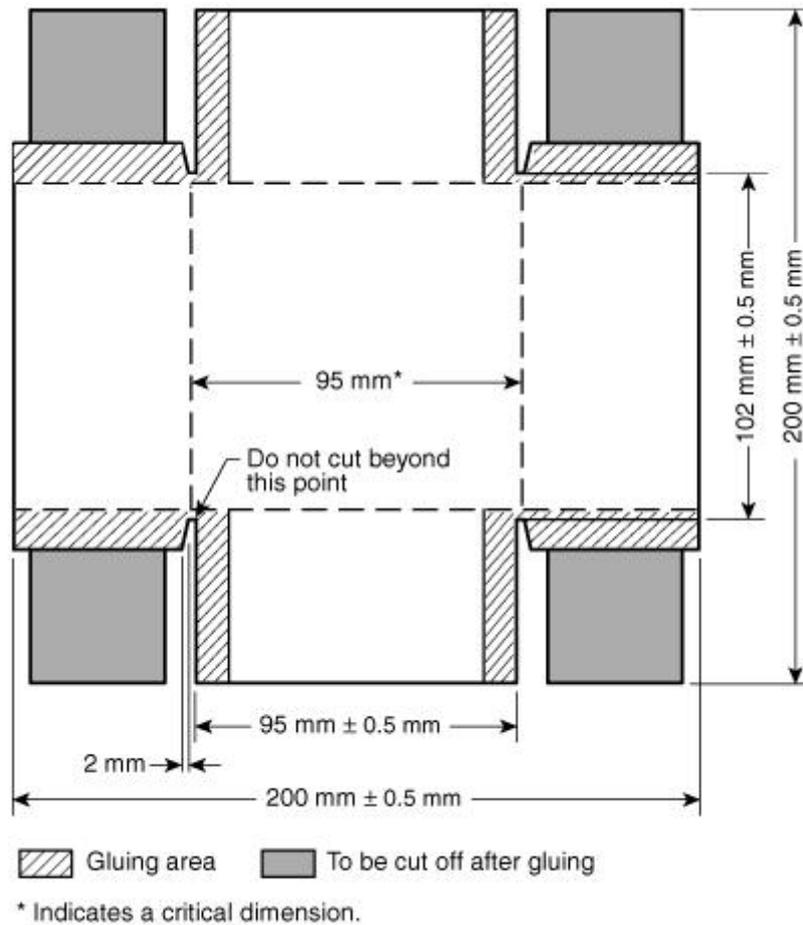
**FIGURE 5.2.8.6(A) Fabric Cutting Shape.**
