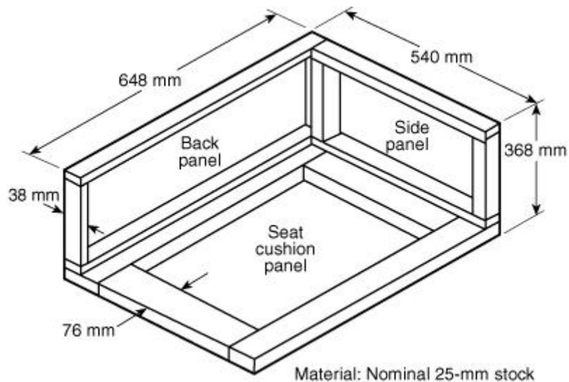
**FIGURE 4.1(a) Frame for Upholstered Furniture Mock-Up Test.**
