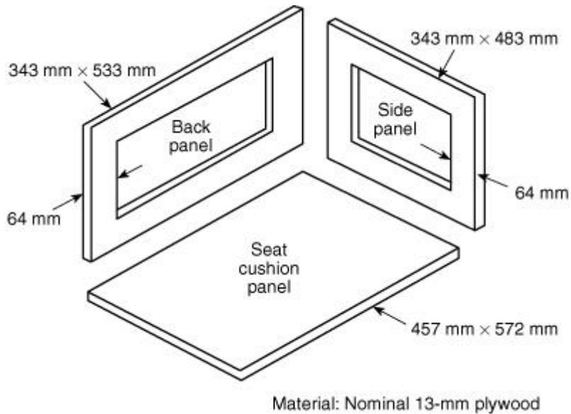
**FIGURE 4.1(c) Panels for Upholstered Furniture Mock-Up Test.**
