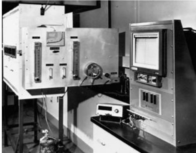
FIGURE 4.1(a) Flooring Radiant Panel Test Apparatus.
