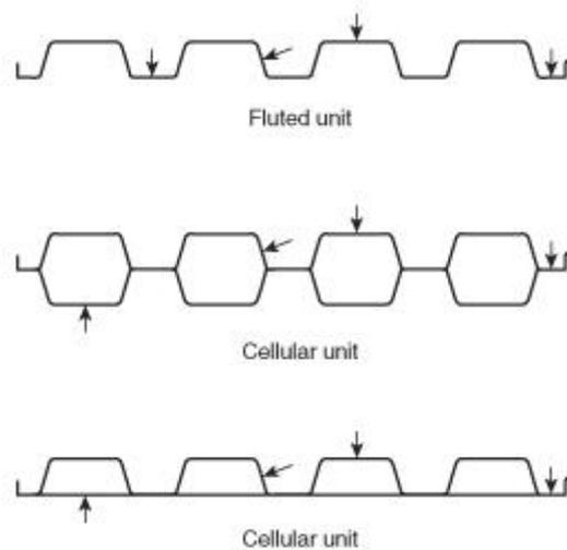
**FIGURE A.11.4.5 Typical Locations of Thermocouples.**
