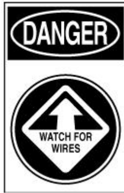
FIGURE 4.1.4.4 Electrical Hazard Warning Label for Fiberglass and Wood Ground Ladders.
