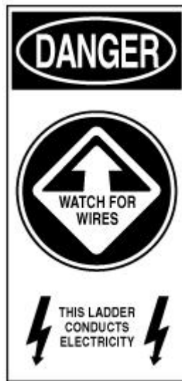
FIGURE 4.1.4.3 Electrical Hazard Warning Label for Metal Ground Ladders.
